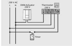
Example of 230V actuator installation with microswitch.
