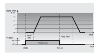
In the auxiliary micro-switch version this is activated following a stroke path of 2mm, as in the below images. At the same time the closure happens after a stroke path of 2mm.
